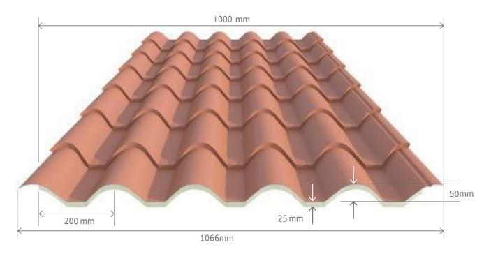
Tile-shaped isothermal panel with high-density polyurethane insulation (55 kg/m³) and aluminum foil on the inside..
